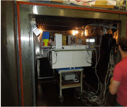
Figure 10: HASP and student payloads in the CSBF BEMCO chamber in preparation for thermal / vacuum testing.
